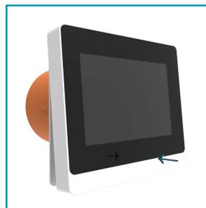
**4.** Fit the front cover to the top of the back cover, then press the bottom of the front cover with your fingers to secure the front cover to the back cover.
